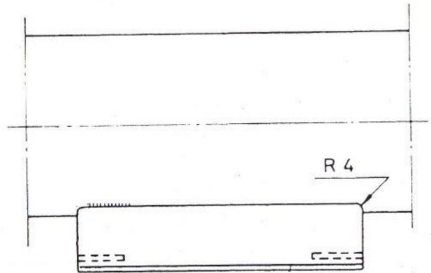
Figure 2 Pipe slide DN 200...500
